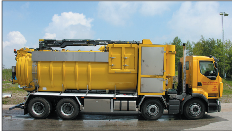
This unit has a 14 m 3 tank and is built on a 4-axle truck chassis
